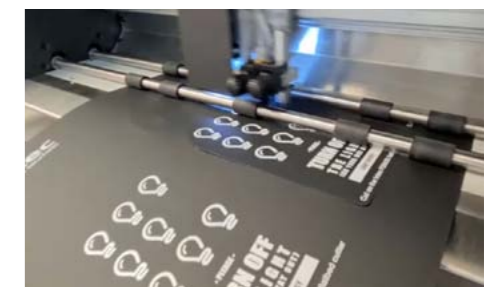
Vision3 camera reads black or white QR codes to instantly retrieve associated cut files
