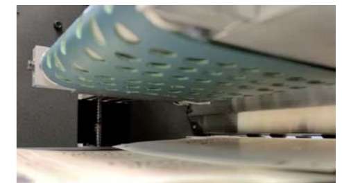
Continuous vacuum belt lifts and feeds sheets onto cutting bed ready for cutting
