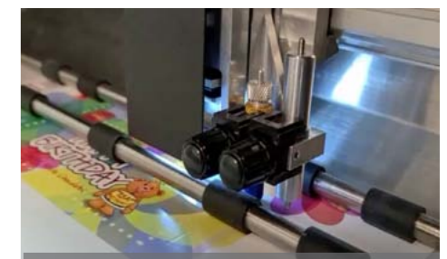
Dual tool cutting with dual grip feeding and revolutionary cutting strip gives perfect results
